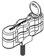
**LOX T-Handle:** Enables security by incorporating a locking mechanism into the handle, preventing anyone from removing your Fuel Pack without having the key.
