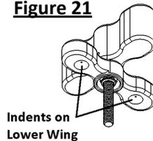
aligned with the bumps on the Fuel Pack (see **Figure 22**) until the Extension Handle is sufficiently tight and the Upper Handle and Lower Wing are perpendicular to each other (see **Figure 23**).
